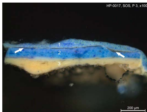
Fig. 4. Paint cross-section of a sample taken from the blue enamel of the Order, showing a separation between the two blue layers.
